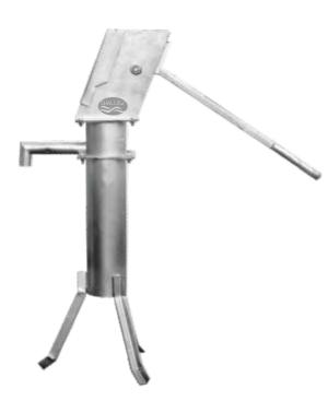
Available Quality & Weight: Light (approx 24 kgs) Medium (approx 29 kgs) Heavy (approx 34 kgs) Super Heavy (approx 39 kgs) Available Colour: Grey colour, Zink Coating, Hot Deep Zink Section Capacity: upto 20 to 45 mt (approx 148 feet) in Borewell Material used: M.S. Material or G.I. Height: 54 inch (approx) Brand: GEC Extra components: Connecting Rods (12 mm 3 meter length), G.I Riser Pipes, (32 mm NB meter length), Cylinder Assembly with All Components.
