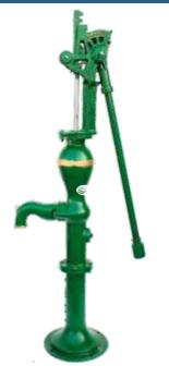
Available Quality & Weight: Regular (approx 24.800 kgs) Available Colour: Dark Green Section Capacity: upto 180 feet (approx) Material used: Casting material (Grey cast iron) Height: 48 inch (approx) Brand: GEC Packing: Single Loose or Wooden Box Pack (Extra Chargeable) Extra components: Connecting Rods (10mm with 3 meter length) G.I Riser Pipes (32 mm NB with 3 meter length) Cylinder Assembly with all Components.
